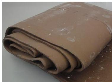
**Figure 1.** First REWASTEE multifunctional material (made of 70% EAFD).
