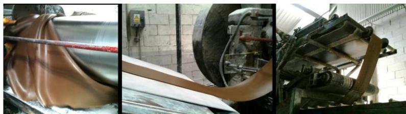
Batch-Off of the REWASTEE Membrane at Trimdelson Trade S.L.
